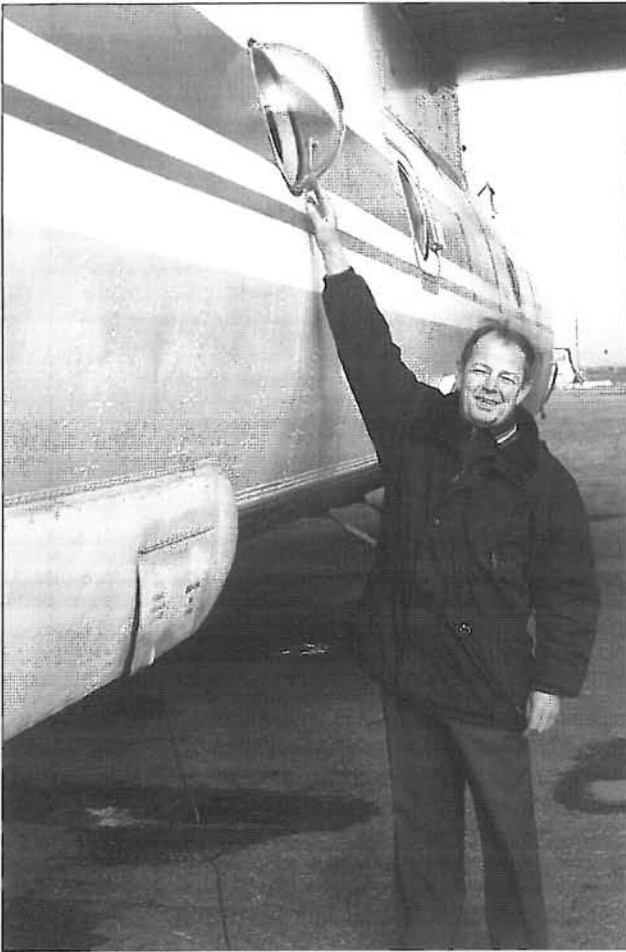
The AN-26 BRL has been modified to be suitable as a platform for observations and for oceanographical work. This includes blisters on both side of the aeroplane. Photo: Hallvard Strøm.
