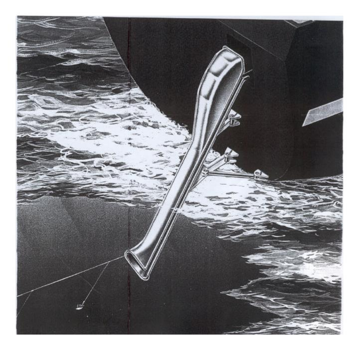
below the water surface. It is manoeuvred hydraulically on hinges from its stern-facing operational setting position to stowing ('parking') position against the hull. The setting pipe or funnel is of sufficient diameter to allow the line (with hooks) to pass down it and exit, while having a slot running the length of the side for external deployment of buoys, weights etc.
